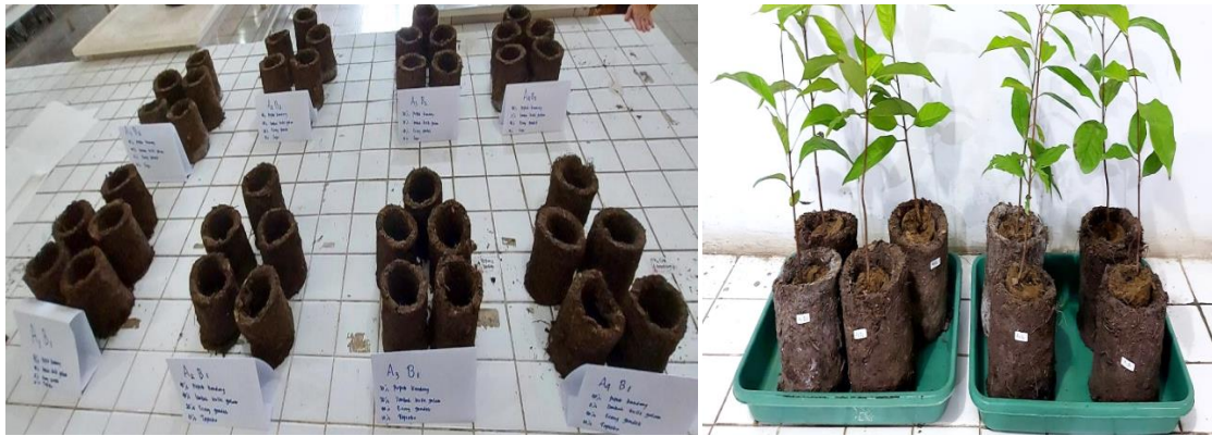
Figure 1 – Organic pot mixed galam skin waste, water hyacinth and manure with the addition of sago and tapioca adhesive
