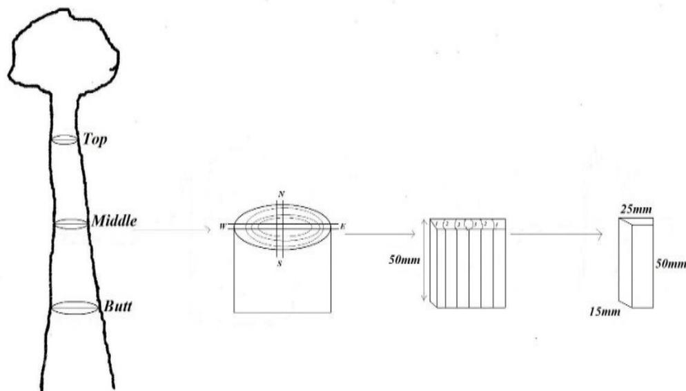
Figure 1 – Schematic diagram showing specimen extraction
